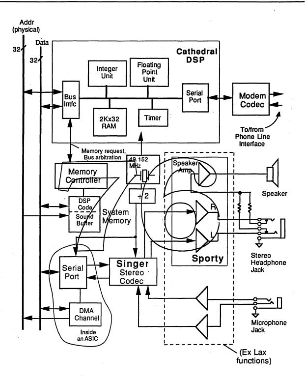
Fig. 14.6 – Sound Hardware for Cathedral-based Machines
