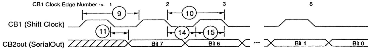
Note that when the Shift Register is programmed to shift out, the falling edge of CB1 is the active edge.
