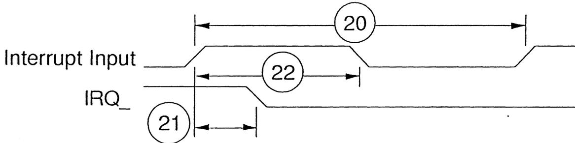
NOTE: Interrupt Input refers to either CA1, CA2, CB1, or CB2. Although timing spec #20 is shown with the rising edge of the Interrupt Input, it should be understood that this timing spec also applies when the falling edge is the active edge. Also note that timing spec #21 assumes that interrupts have been enabled for the particular Interrupt Input in question, otherwise IRQ\_ would not go active. Timing spec #22 specifies the minimum pulse width for active high and active low pulses.
