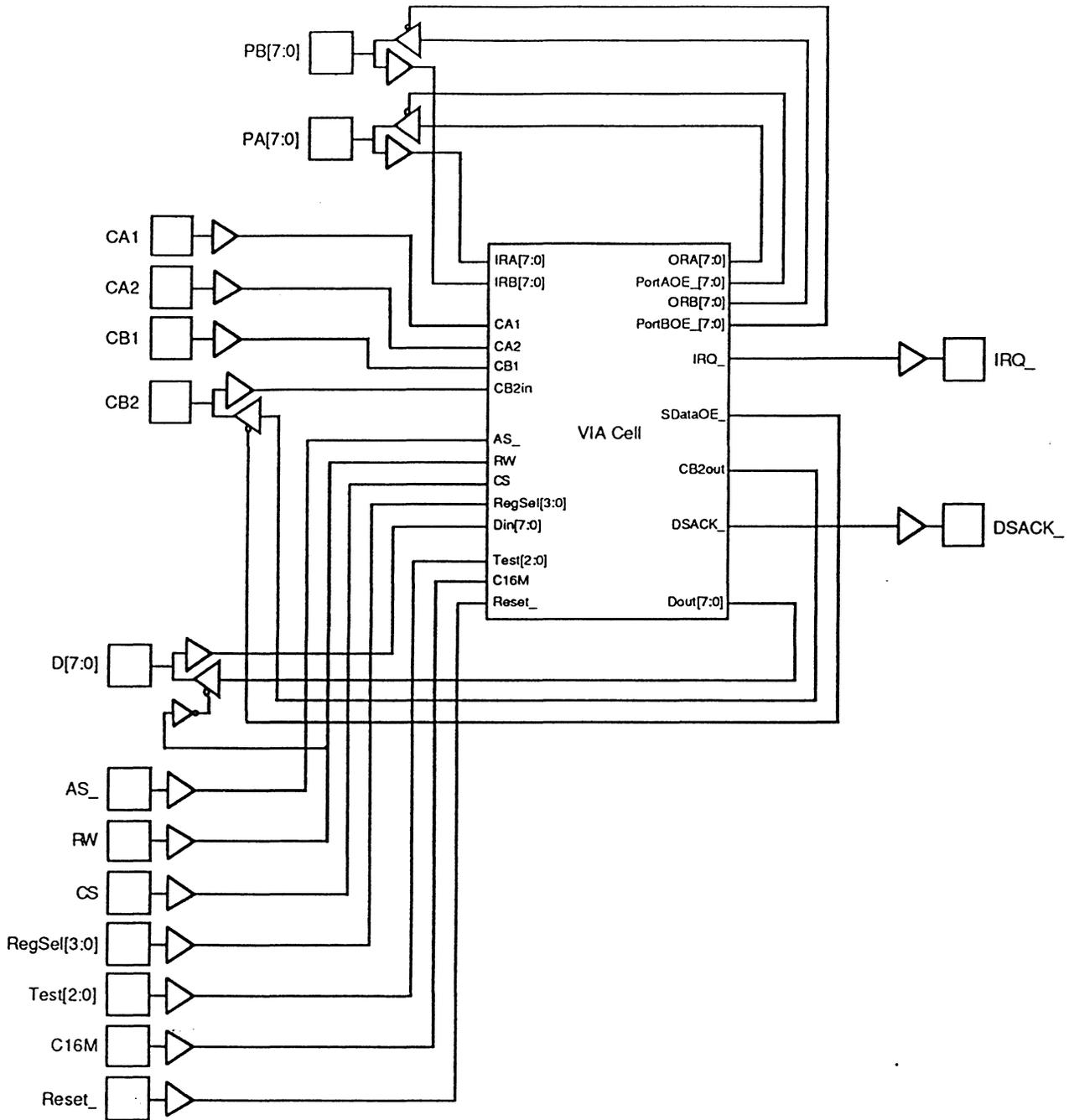
Figure 17 - Using the VIA Cell within a Larger Chip
