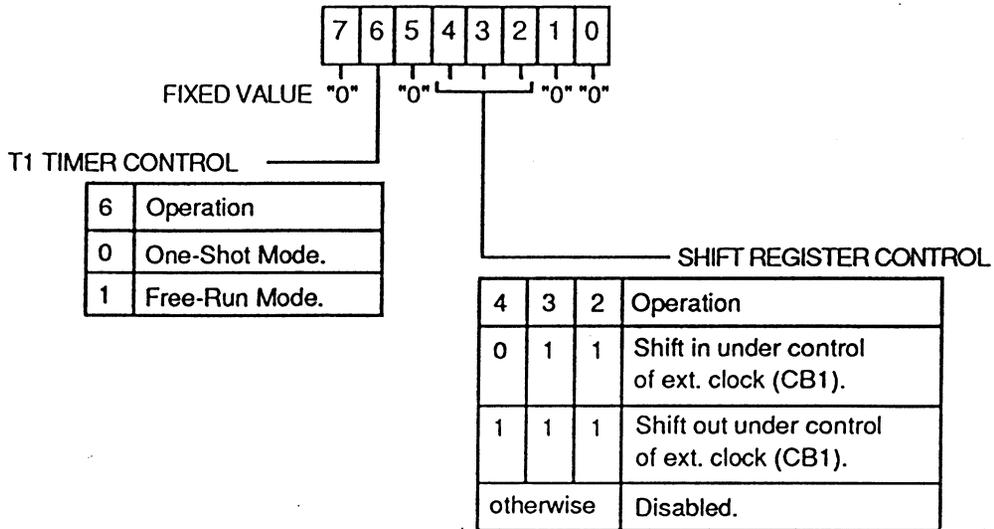
Note that bits 7, 5, 1, and 0 of the ACR are hardwired to "0". These bits are used in the 6523 VIA to select modes which are not supported in the VIA Cell.
