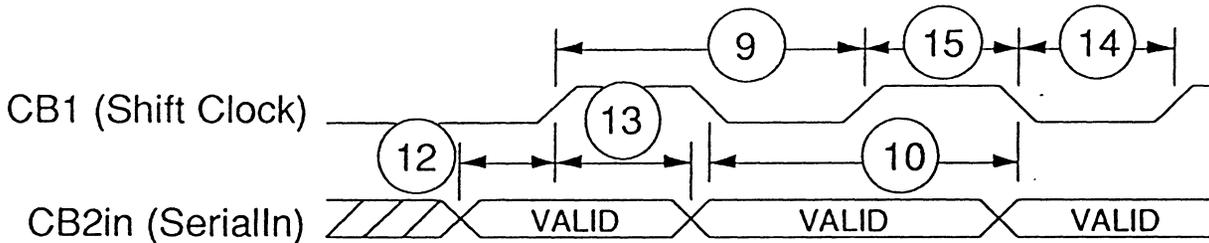
Note that when the Shift Register is programmed to shift in, the rising edge of CB1 is the active edge.
