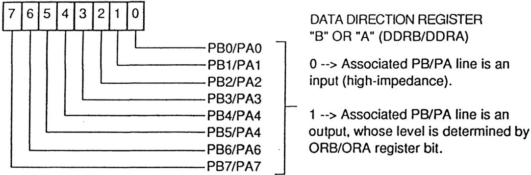
Figure 4 - Data Direction Registers (DDRA, DDRB)
