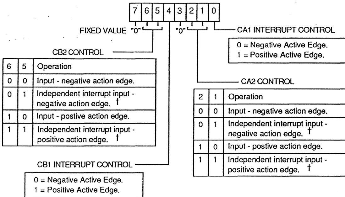
† If the CA2/CB2 control in the PCR is selected as an "independent" interrupt input, then reading or writing Port A or Port B will not clear the corresponding Interrupt Flag Register bit. Instead, the bit must be cleared by writing into the IFR, as described previously.
