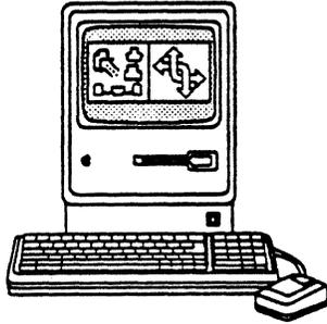
Under most circumstances, an AppleTalk Internet Router should *not* be run on a Macintosh computer that will be used concurrently as a user's workstation. User activities might require shutting down or restarting the system, or might lead to system errors that would interrupt router operation. In addition, user applications on the workstation would suffer from reduced performance due to router processing.
