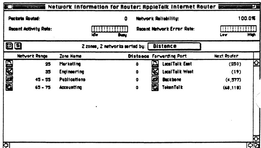
The routing table is the foundation of the logic that makes internet routing possible. It is the logical map of the internet that the router uses to forward packets between networks through the most direct route.
