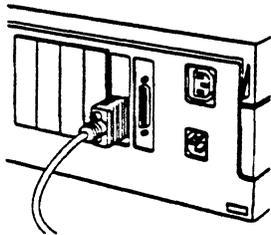
Each Macintosh computer is equipped with two standard serial ports: a modem port and a printer port. Both of these ports are used for network connections when the AppleTalk Internet Router is set up as a LocalTalk-to-LocalTalk router.
