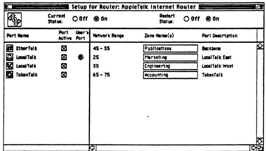
The Router Setup window presents one line for each possible network connection. The number of lines displayed is determined by the number of AppleTalk network ports installed in the Macintosh.
