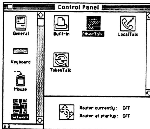
Control Panel resource files produce icons in the Control Panel (for example, the Keyboard and Mouse icons) that allow you to display the corresponding options and settings for these resources.
