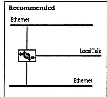
When connecting networks of different speeds, consider that the router does not distinguish the speed of a network when selecting a route to a destination; it favors the route with the least number of hops.
