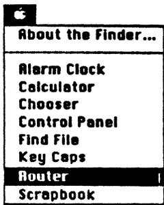
The Router desk accessory appears in the Apple menu after installation of the router software.
