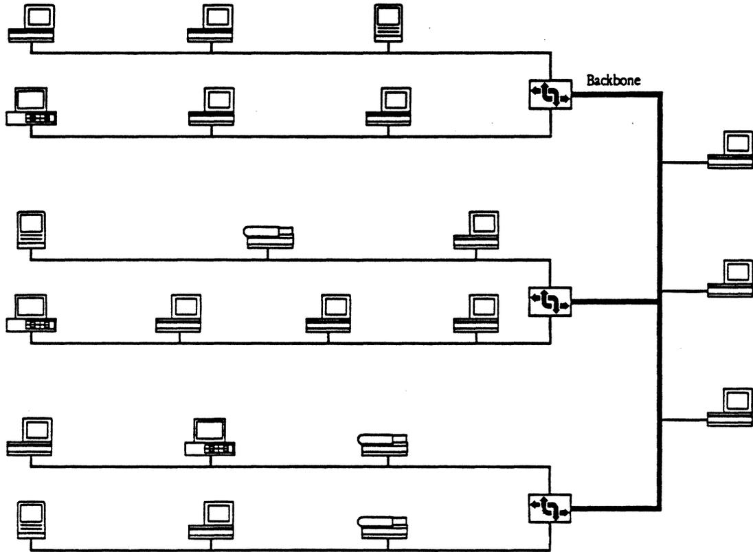
If a break should occur on any individual network (other than the backbone), other networks can maintain uninterrupted communication, independently of the inactive network.
