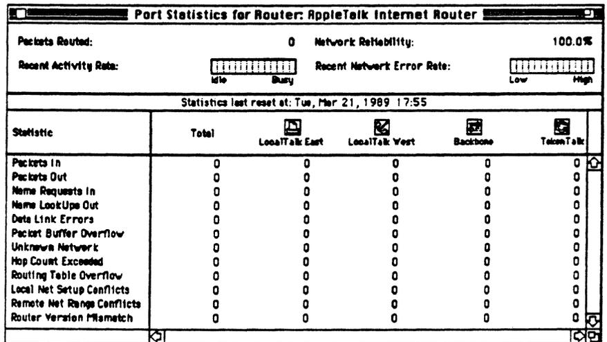
The statistics are listed separately for each individual port, so you can monitor relative activity and error levels of connected networks.
