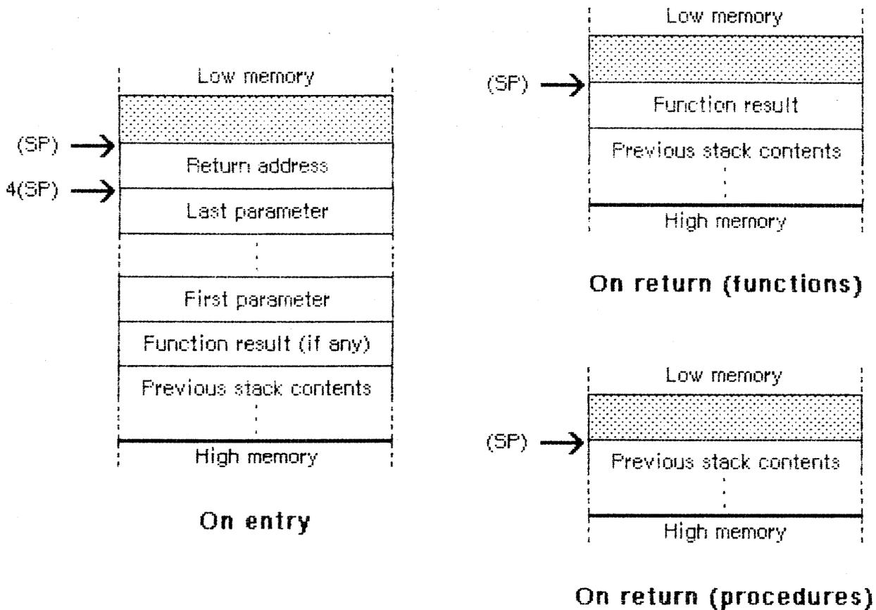
Figure 5. Stack Format for Stack-Based Calls
