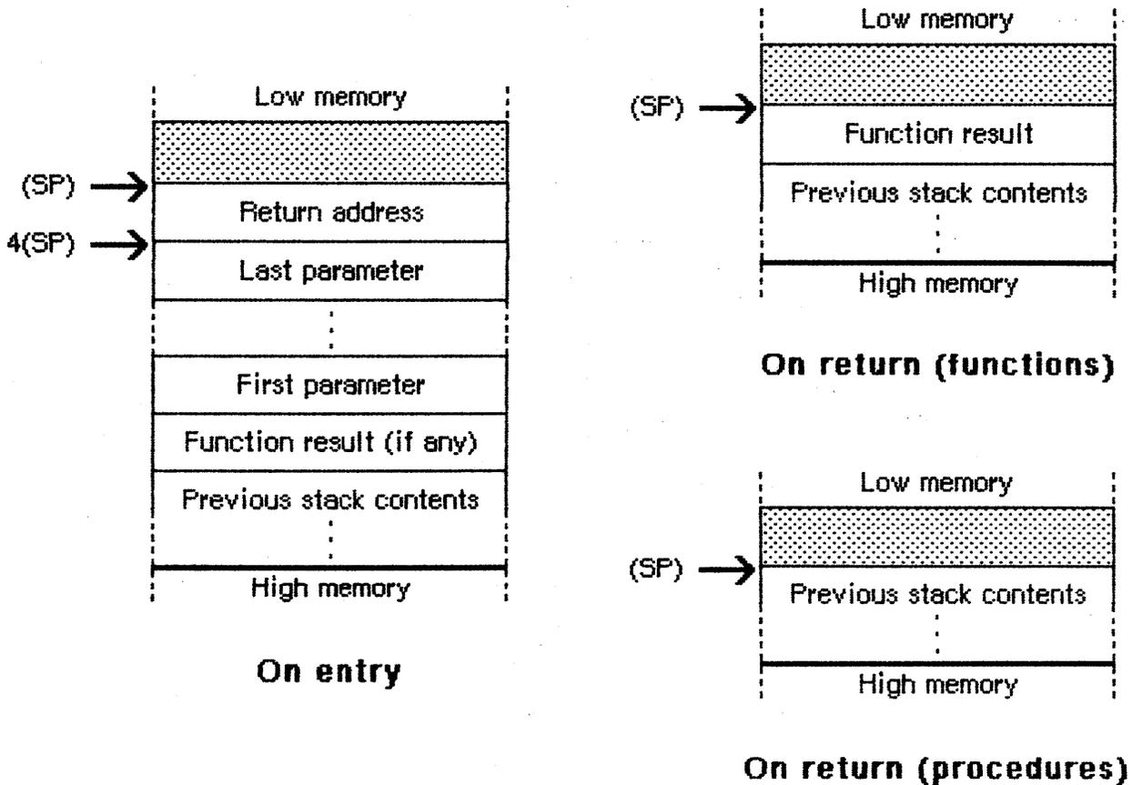
Figure 5. Stack Format for Stack-Based Calls
