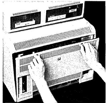
6. Determine which of the three expansion slots on the lower left of the card cage will hold the card.
