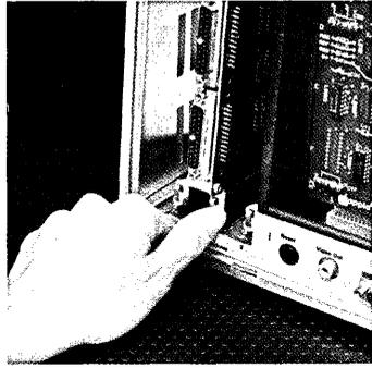
12. A set of slot covers on the Lisa's back panel blocks the electromagnetic emissions from inside the cabinet. If you have just installed a card into a slot that did not previously contain a card, follow steps a through e for removing the cover that protects that slot.
