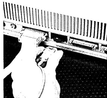
4. Remove any cables extending from the expansion cards on the left side of the back panel.
