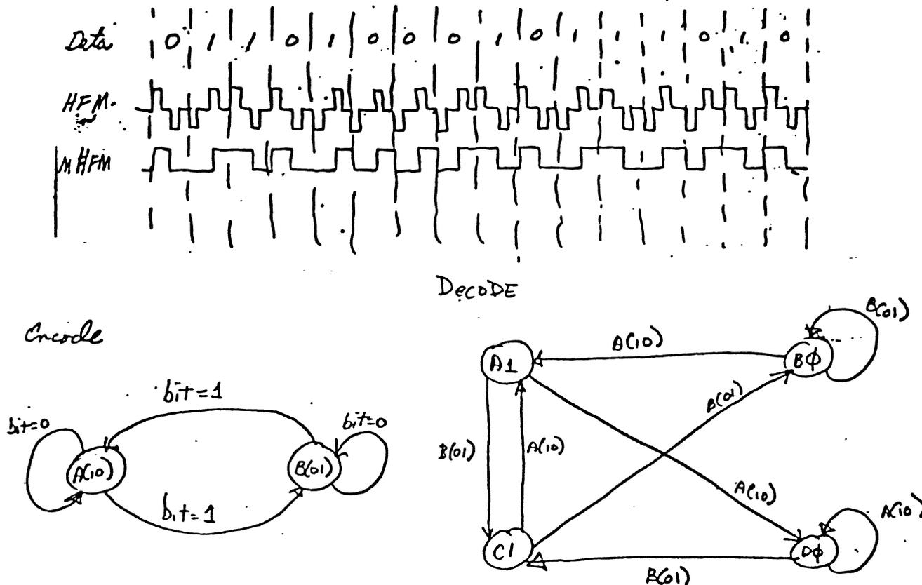
Figure 2-2. MHFM and HFM Transmission Codes.
