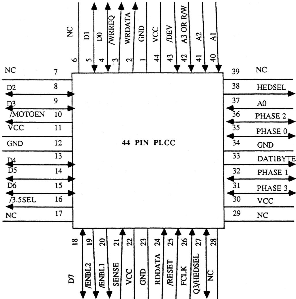
PHASE 0 - PHASE 3 - These lines can be programmed to be either inputs or outputs, and are used for communication with the disk drive.
