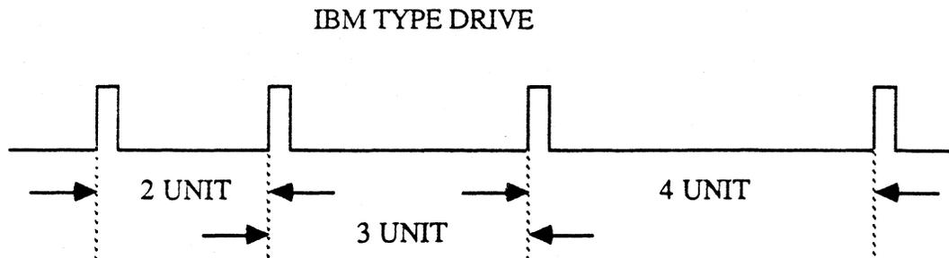
Therefore a mode is added to the chip which makes it possible to get this type of Wrdata signal, so that it can be made possible to deal with both types of drives. This can be accomplished by delaying the the toggling Wrdata pulse, that is already generated, by 4 clocks when not Long (when not shifting by an extra half clock) or by 4 1/2 clocks when Long (extra half shift is desired).
