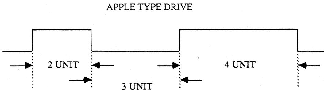
This data pattern to the disk works fine for Apple standard drive, but for IBM type drives the wave form needs to consist of pulses spaced at 2, 3, and 4 units apart.
