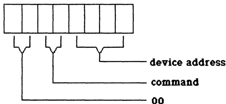
Note that the defined advanced commands have the two most significant bits set to "00".
