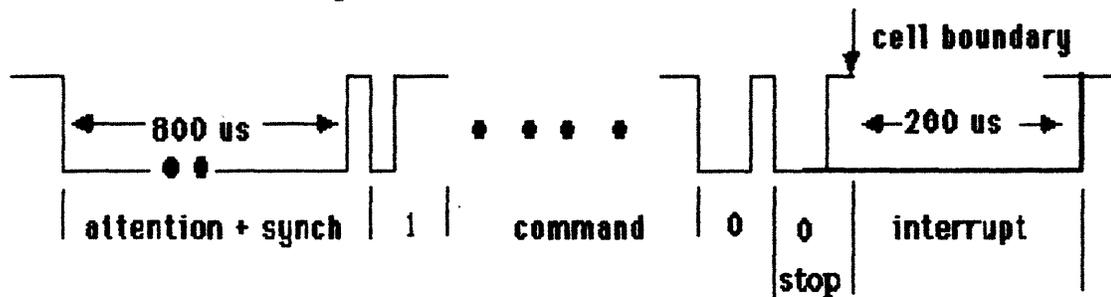
The **RESET** signal has the effect that it resets all pending interrupts; it turns the interrupt mode of all devices to **DISABLE**; and in general puts the devices in a mode in which they will accept commands. **RESET** issues a break on the bus by holding the bus low for a minimum of 2 ms.
