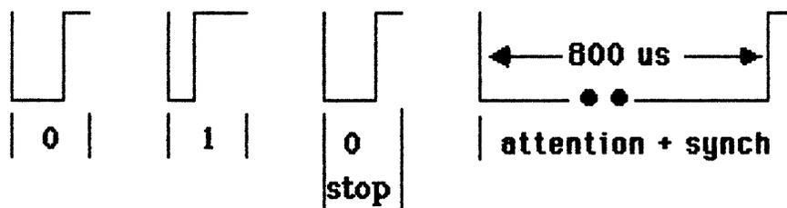
As a specific example, a **TALK** command to register 0 of device 6 would be encoded as "11000110". The bus would be modulated with the following:
