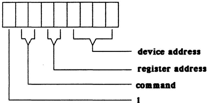
Note that the MSB of all commands is set to "1". Only the bus master has the ability to drive the MSB of any transaction on the bus to a "1". Conversely, all data transactions have the MSB set to "0". The bus master as well as any other device on the bus has the ability to set the MSB to "0".
