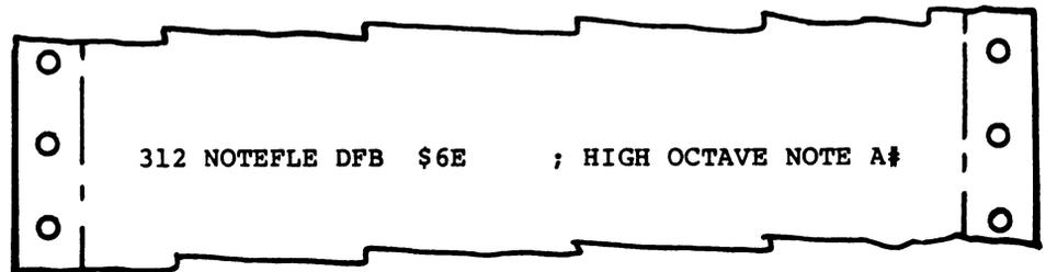
. . . puts the value hexadecimal \$6E into the file whose starting address equals NOTEFLE. The operand here can be in hex, in decimal, or can even be a label. Whatever you use, the operand must be convertible to an 8-bit data value ranging from hex \$00 to \$FF, or from decimal 0 to 255. Sometimes you will put a label on each file entry, while other times you just name the base address at the start of the file.
