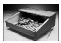
The original Apple I (shown here in a custombuilt wooden case) was little more than a circuit board to which customers were expected to add a case, power supply, monitor, and keyboard.
