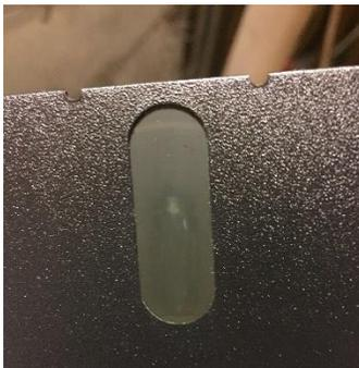
Figure 5: Media damage from removing adhesive
