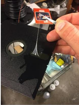
Figure 3: Adhesive removed from jacket but still adhered to media surface
