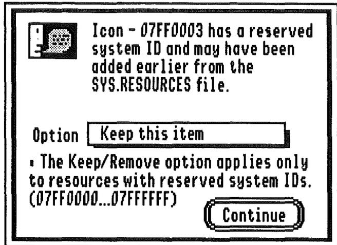
Figure 2-6 *Option Window Presented When a Resource Numbered in the System Range Is Encountered by Optimize File*
