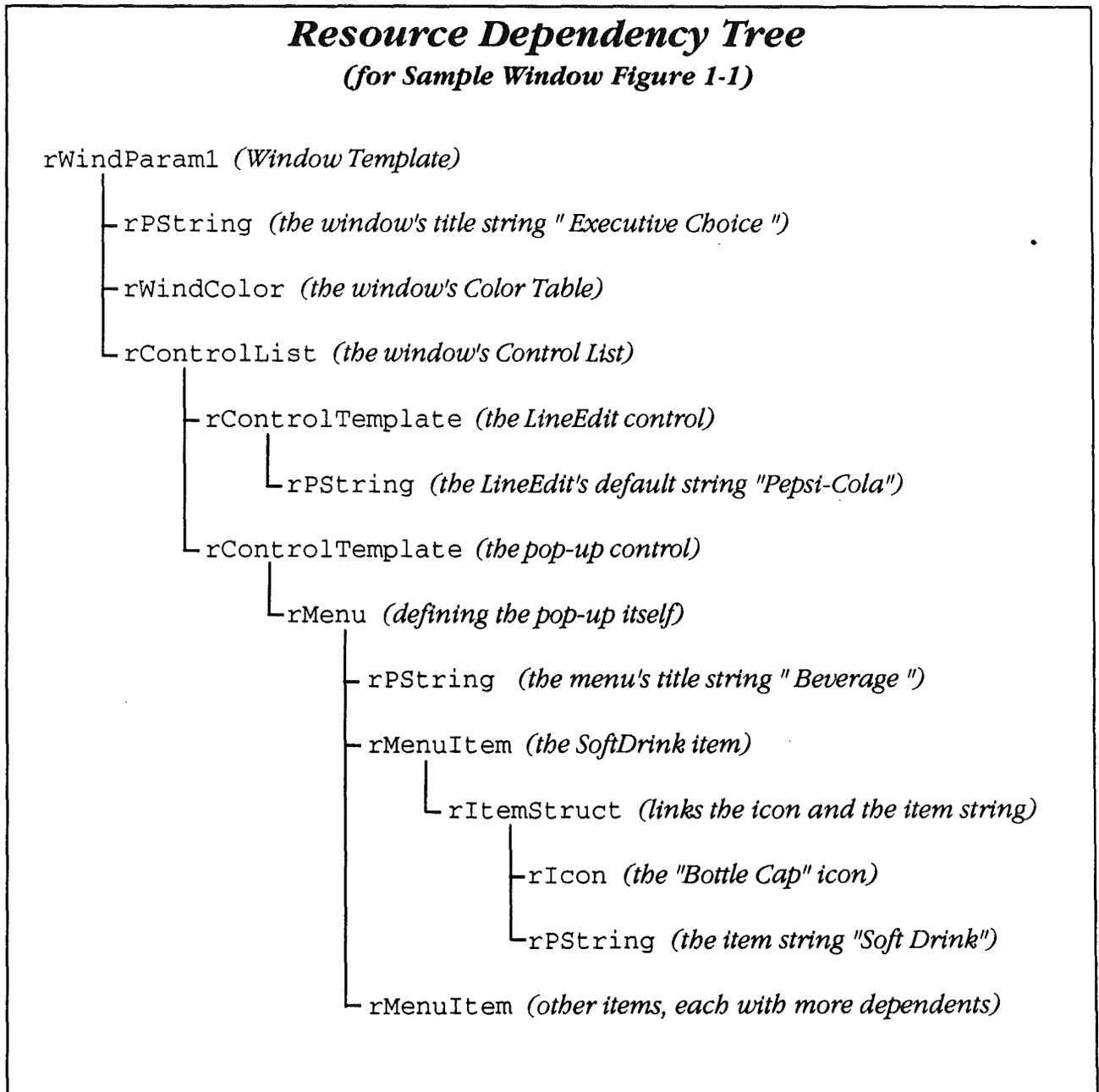
Figure 1-2 Diagram illustrating the Sample Window resource dependency structure
