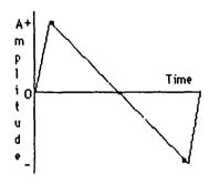
From the two points sampled, the sawtooth could be (more or less) accurately drawn. The upshot of this, however, is that for a sample of at least two points per waveform to be passed to the digital-to-analog converter, the waveform must be sufficiently low (or slow) for the two points to be passed. A case in point is a fre-
