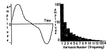
The waveform depicted above is typical of a sawtooth containing twenty harmonics. As we add more harmonics, the wave approaches a perfect sawtooth, without the slight perturbations seen in the model. An instrument such as the violin would, in fact, produce up to fifty or sixty harmonics within a single tone. Unfortunately, here is where the first of our problem areas is encountered.
