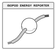
The isopod snaps onto one of your your incoming power lines right at your weatherhead. This is basically a self-powered current transformer and a short range transmitter.
