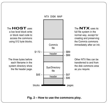
works: A host computer with any old SCSI driver is connected to one or more SCSI hard disks. Your last hard disk in your chain also gets connected to a SCSI PostScript laser printer such as a *LaserWriter NTX*. Priorities are established so that the laser printer is the boss.
