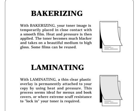
Fig. 2 - Two methods to improve toner durability.
