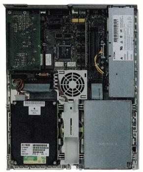
Mac LC logic board; Ile Card installed, top left.
