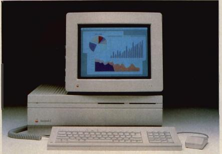
The Macintosh II looks nothing like a Macintosh. Its separate system unit and display make it appear similar to the Apple IIGS. This Mac II is equipped with the optional color display.
