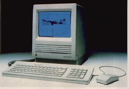
The Macintosh SE—a faster version of the Macintosh Plus—offers limited expandability, an optional internal hard drive, and choices in keyboards. Note the 81-key keyboard pictured here.
