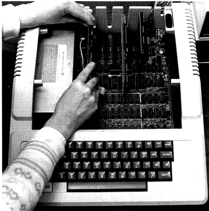
Inserting the RAMCard Memory Board into Slot 0
