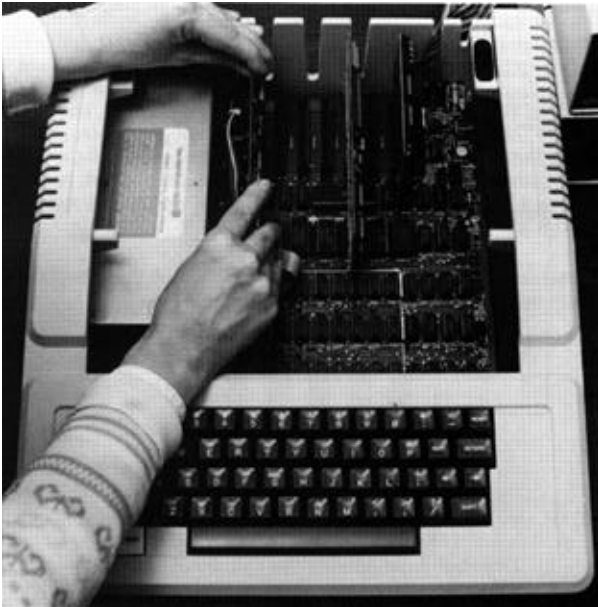
Inserting RAMCard into Slot 0
