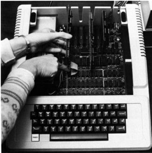
Inserting the RAMCard Cable
