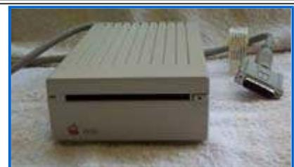
It was designed for use with Macs with an FDHD disk controller (eg SE FDHD, SE/30, IIX, IICi). If used with a Mac that doesn't have an FDHD controller, it will operate as an 800K drive. It should not be used with the Mac 128K or 512K.
