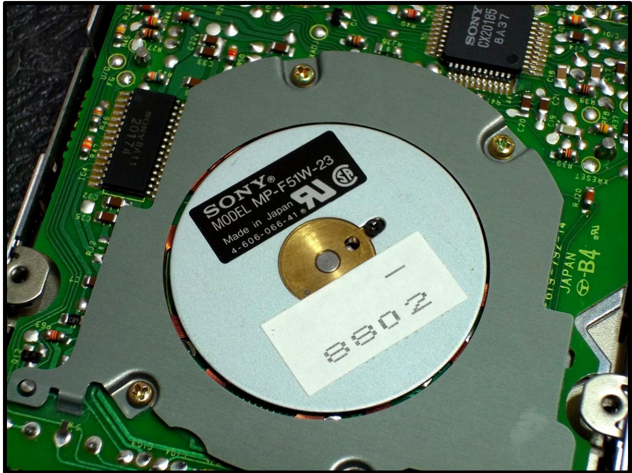
Figure 4. The Sony 3.5 floppy disk drive mechanism used in the Apple 1.44 Mb floppy disk drives.
