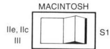
Figure 2-5. Rocker Switch Settings (Apple //c)
