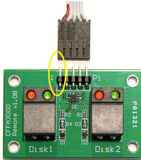
Figure 12: CFFA3000 Remote connector P1 pin 1 location
