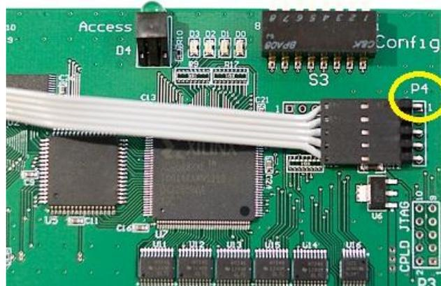
Figure 14: CFFA3000 connector to remote P4 pin1, oriented forward
