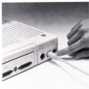
Figure 1. Turning Off the Apple IIc
