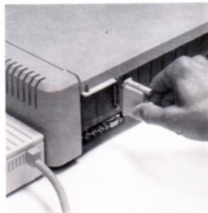
Figure 9. Plugging the UniDisk 3.5 Into an Apple IIe.
