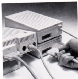
Figure 10. Connecting a Disk IIc Drive.
