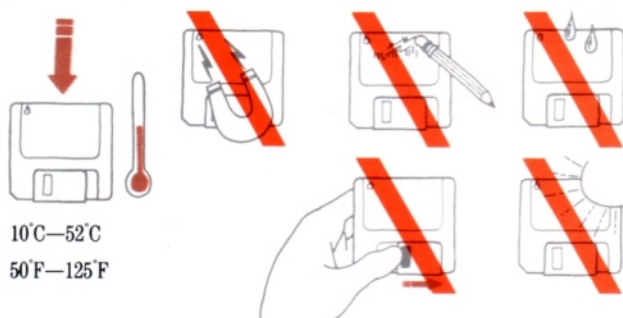
Figure 17. Care and Handling of 3½-Inch Disks
