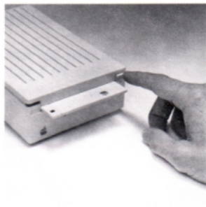
Figure 14. Ejecting a 3½-Inch Disk.
