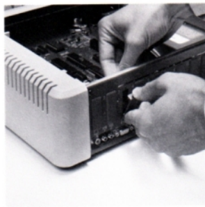
Figure 5. Removing the Cover Plate From an Apple IIe
