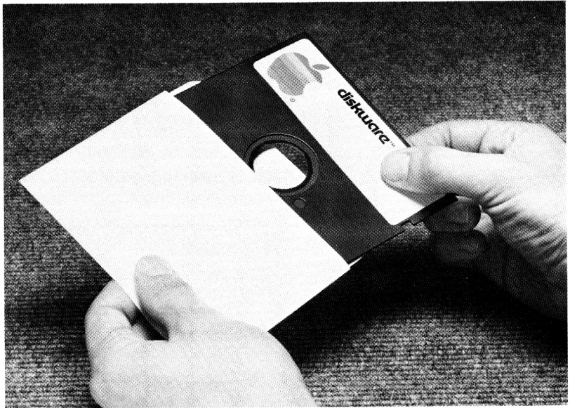
Figure 3-4. Removing a Disk From its Envelope
