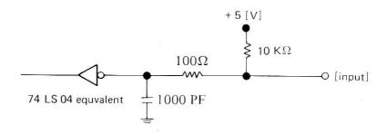
The  $\overline{STROBE}$  and  $\overline{INITIAL}$  signals are pulled up to +5.0 [V] with a 1000 ohm resistor. One hundred (100) ohms and 1000 PF are added to the  $\overline{STROBE}$  and  $\overline{INITIAL}$  signals only.
