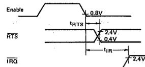
Figure 6 RTS Delay and IRQ Release Time
