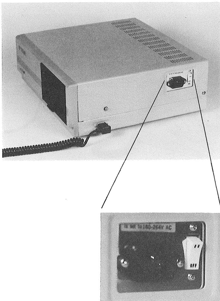
**FIG. 2-3** Power switch in OFF position
