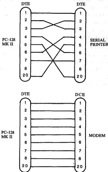
**FIG 17-1 (a) Connecting to a serial printer
