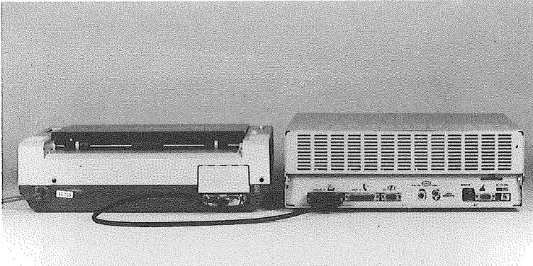
*FIG. 2-14 Connecting a printer to the System Unit*
