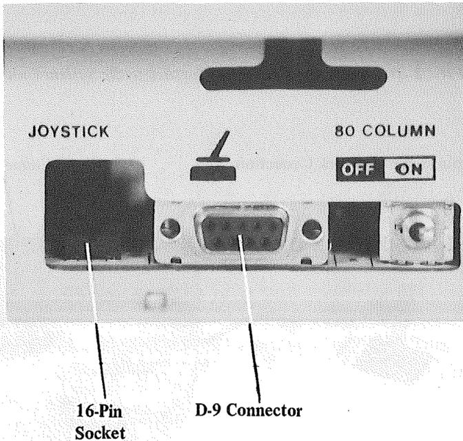
*FIG 2-15 Two types of joystick connector*
