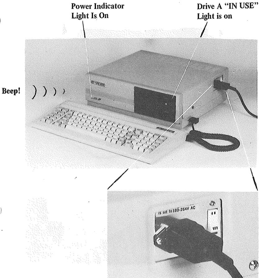
*FIG. 2-5 The responses of the System Unit during the test*
