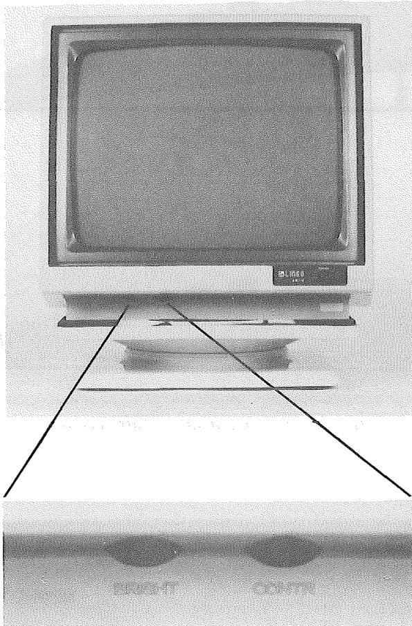
*FIG. 2-21 Adjusting the contrast and brightness of the monitor*
