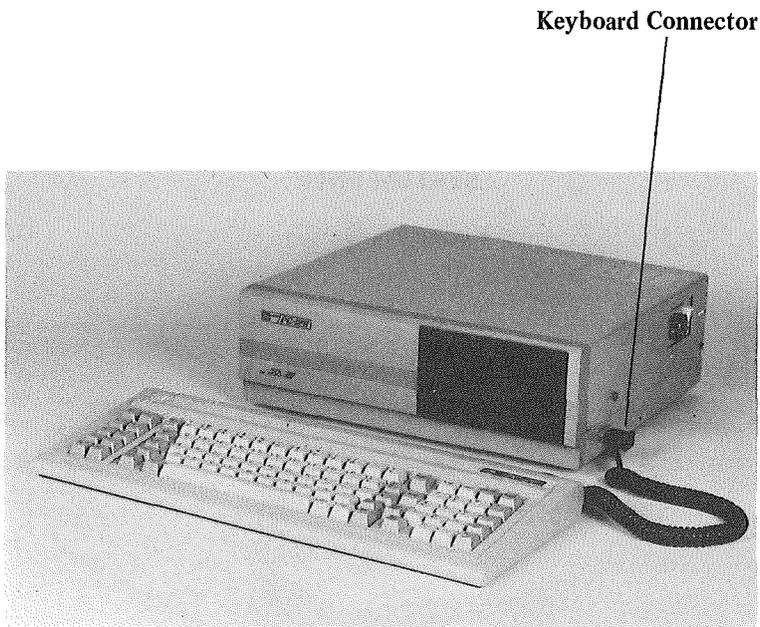
*FIG. 1-2 Connecting the keyboard to the System Unit*
