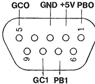
**FIG 14-1 Game I/O Connector Pinout**
