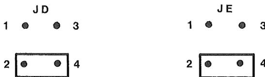
*FIG 18-3 Serial slot 1, Parallel disabled*
