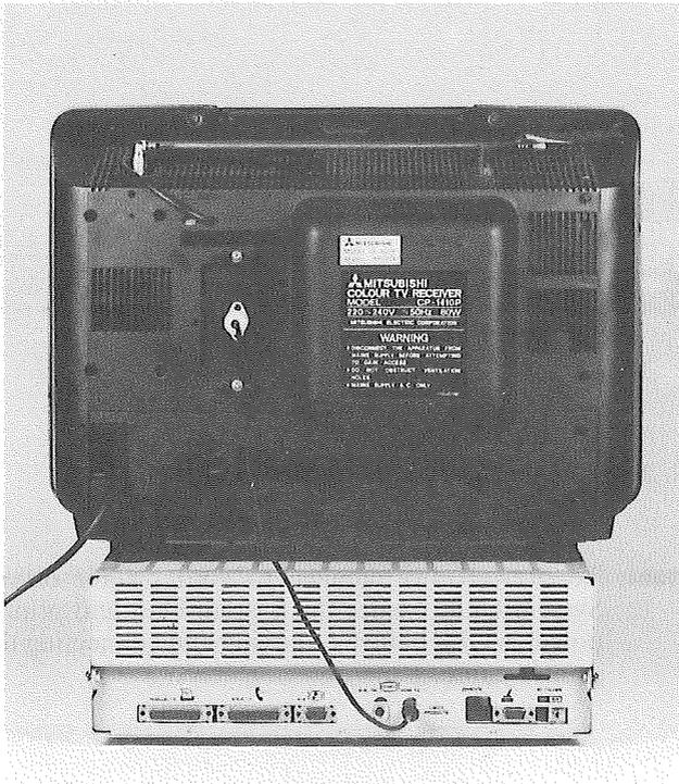
*FIG. 2-13 Connecting a TV to the System Unit*
