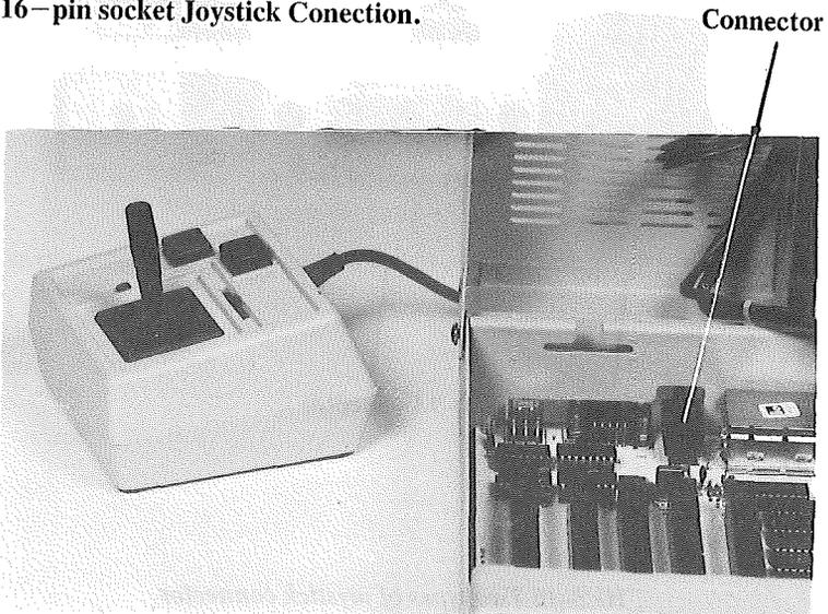
*FIG. 2-17 Connecting a 16-pin type joystick to the System Unit*
