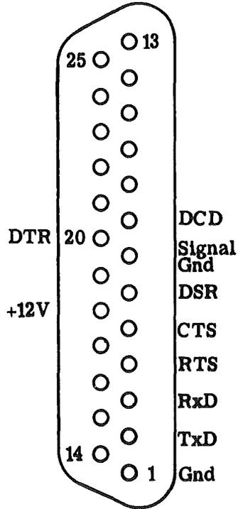
*FIG 17-2 Serial Interface Pinout*
