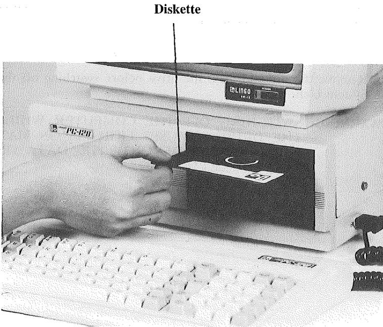
*FIG. 3-4 Inserting a diskette into the drive*
