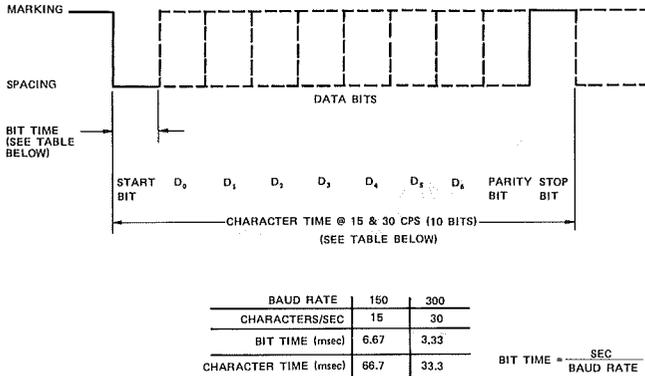
Figure 11 150 & 300 Baud Serial ASCII Data Timing
