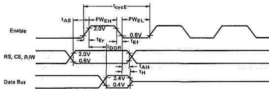
Figure 7 Bus Read Timing Characteristics
