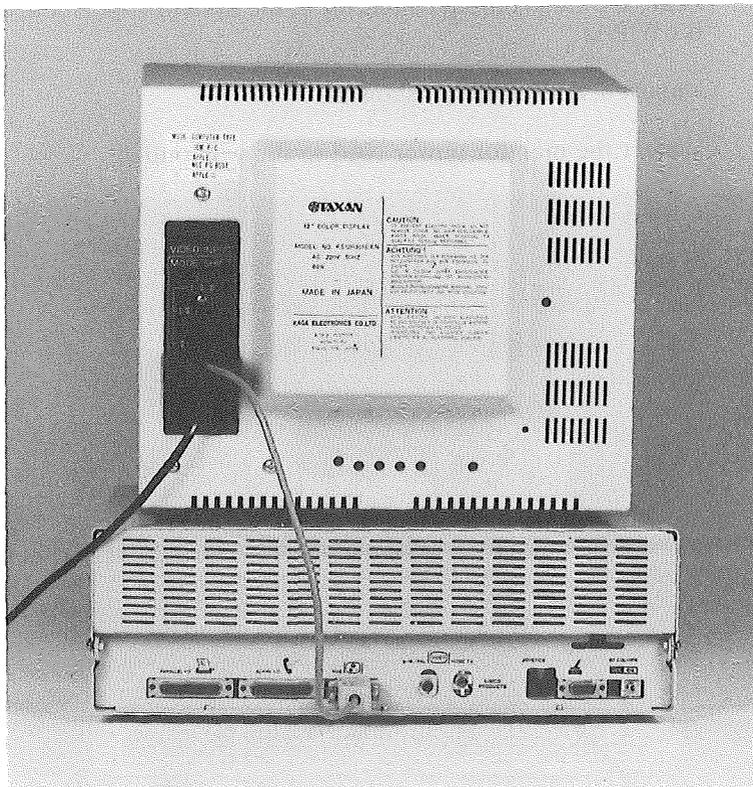
**FIG. 2-12** Connecting a RGB monitor to the System Unit
