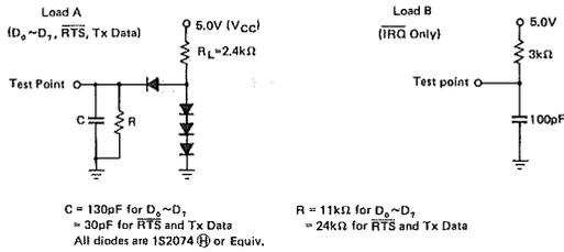
Figure 9 Bus Timing Test Loads
