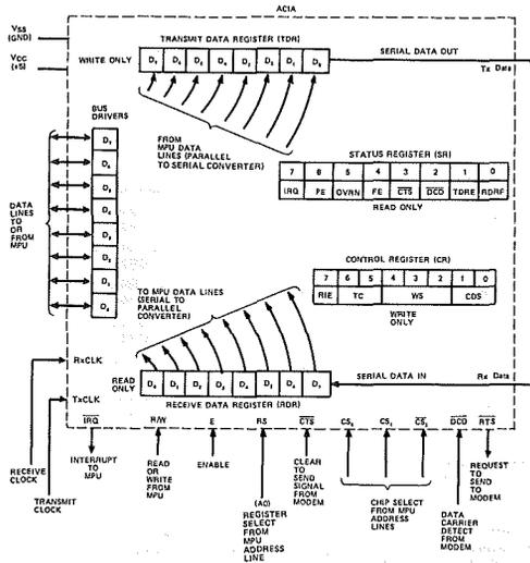
Figure 13 Internal Structure of ACIA
