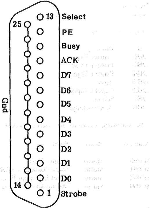
**FIG 16-1 Printer Interface Pinout**
