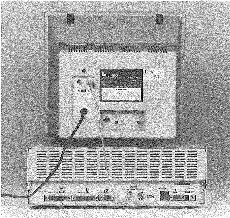
*FIG 2-11 Connecting a monochrome monitor to the System Unit*
