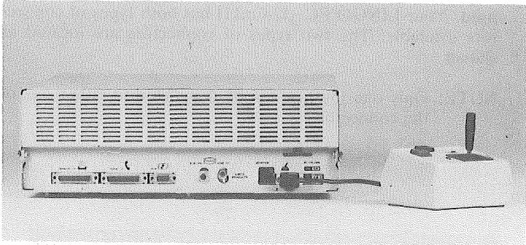
*FIG. 2-16 Connecting a D-9 type joystick to the System Unit*
