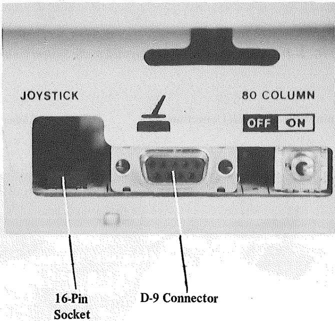
*FIG 2-15 Two types of joystick connector*
