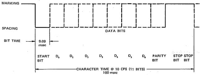
Figure 10 110 Baud Serial ASCII Data Timing
