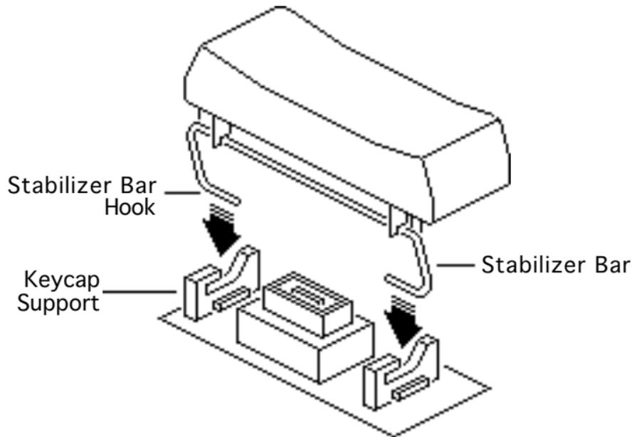
**Replacement Note:** The Spacebar, Delete, Return, Tab, Shift, Enter, and “0” keys use stabilizer bars to secure the keycaps.
