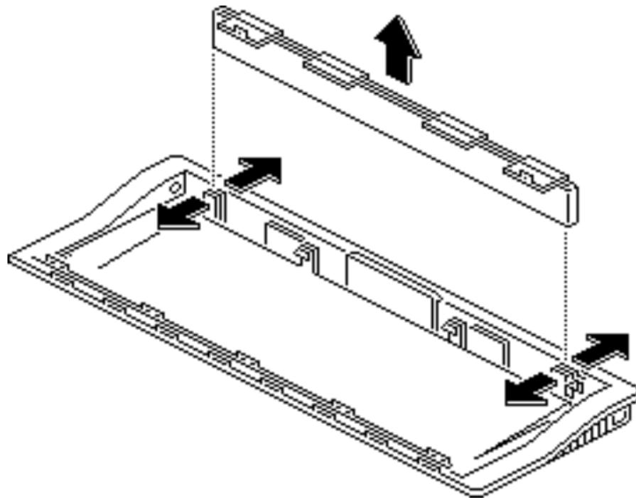
10 Spread the rear foot plastic clips and lift out the rear foot.
