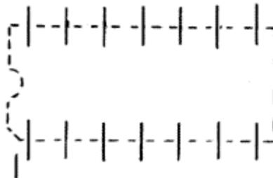
The solid lines on the schematic represent electrical conductors like wires and printed circuit lanes. If there is a dot where two solid lines meet or cross the conductors are connected. If there is a small loop or no dot the conductors do not connect.
