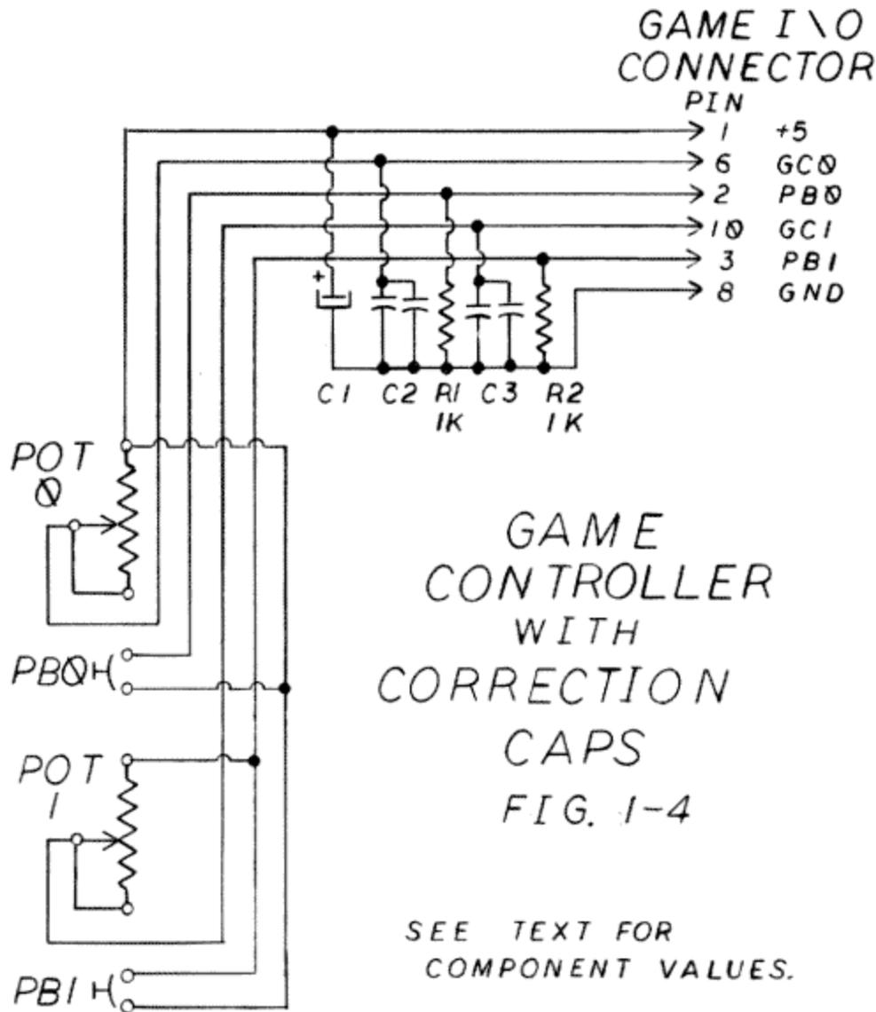
The timing circuit can be adjusted for pot values lower than the original values. This adjustment can be made by adding small capacitors within the paddle and thus requires no modification of the host computer. Figure 1-4 shows how the correction caps can be added to a standard controller circuit.
