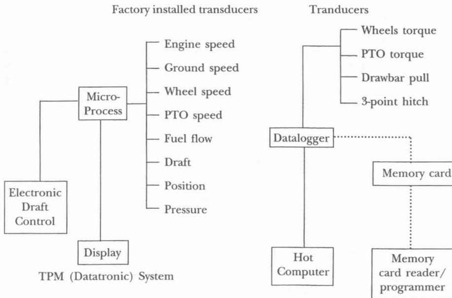
Fig 2. Block diagram of the tractor instrumentation system
