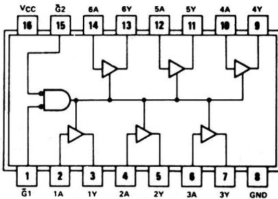
Fig. 6-7. SN74365, or DM8095 three-state buffer chip pin configuration.
