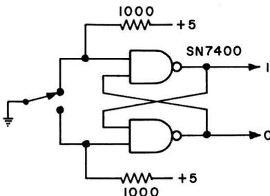
Fig. A-3, two outputs are available. With the switch in the position shown, the normal logic states are shown at the outputs of the two gates. When the switch is moved to the other position, the outputs of the NAND gates will switch. It is suggested that a momentary switch be used in the pulser circuits.
