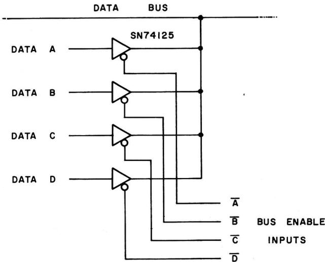
Fig. 3-8. Typical three-state bus for four devices.
