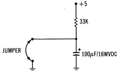
Use the jumper wire to discharge the capacitor, and leave it in place until after you have started the program. Once the program is running, remove the jumper to ground. You should see the voltage slowly increase, as the capacitor is charged. Why does the graph show the zero-voltage point on the top of the screen, and the high-voltage point on the bottom?
