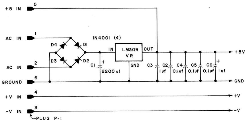
Fig. 5-2. Breadboard power-supply circuit schematic.
