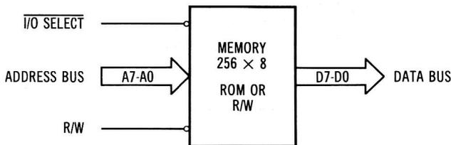
Fig. 7-1. Using I/O SELECT to control a page of memory.
