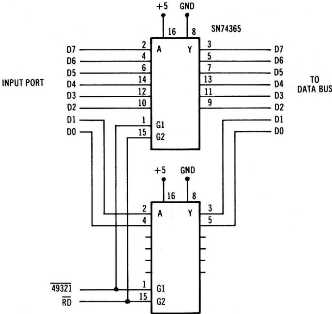
Fig. 3-10. Typical input port constructed using SN74365 chips.
