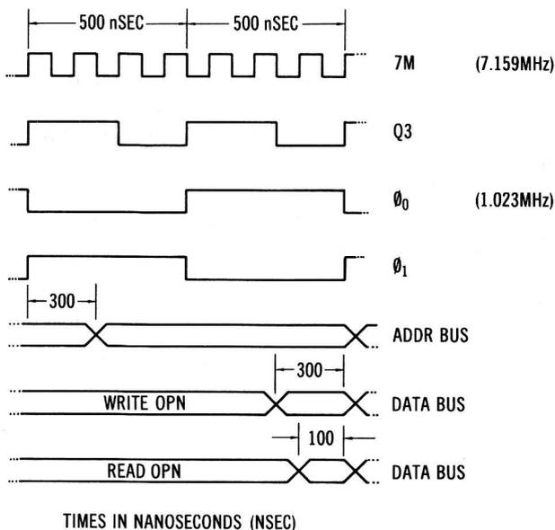
**Fig. 7-8.** Timing diagram for various Apple clock signals.
