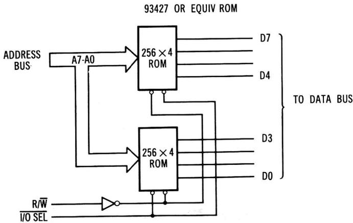
Fig. 7-11. A 256-byte memory expansion circuit diagram.
