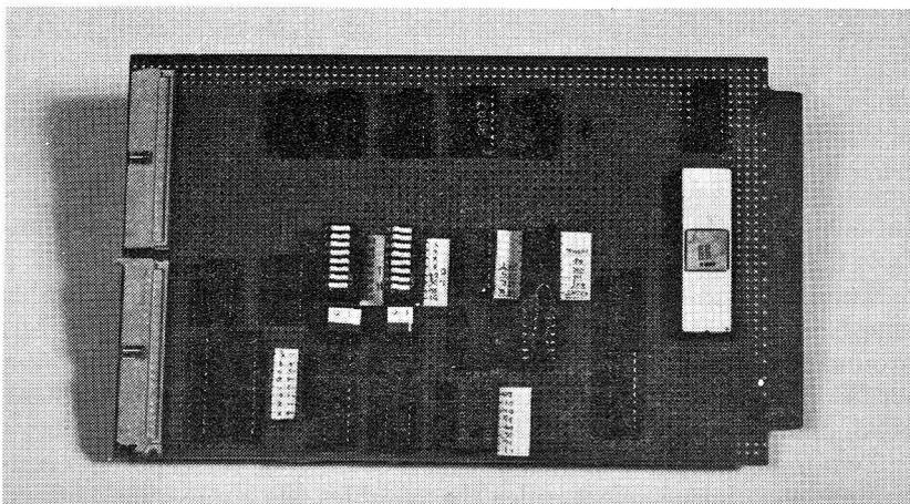
**Fig. 5-9. Wire-wrap version of the interface circuit.**
