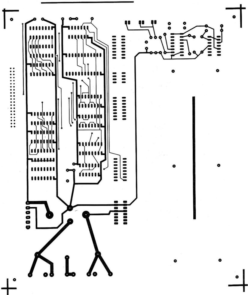
Fig. E-1. Printed-circuit board artwork for component side of interface breadboard (right reading).
