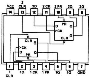
Fig. 6-20. SN7474 dual D-type flip-flop chip pin configuration.
