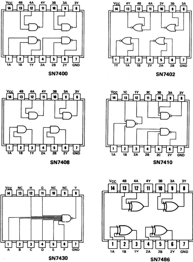
Fig. 6-17. Pin configurations of some standard gates.
