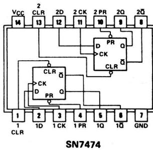
Fig. 6-5. SN7402 and SN7474 chip pin configurations.
