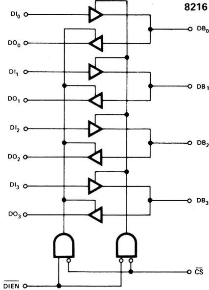
**Fig. 5-6. The 8216 bus buffer chip pin configuration.**
