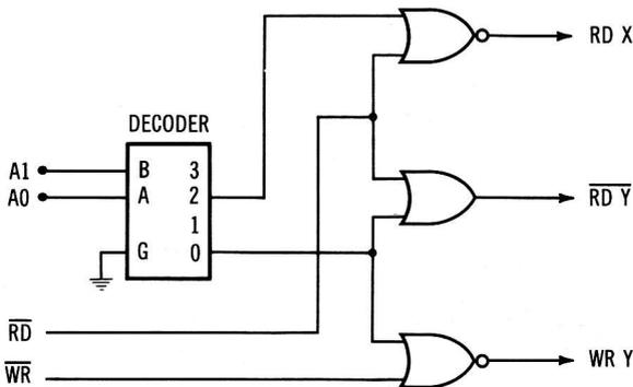
**Fig. 2-8. 2-Line-to-4-line decoder used for device addressing.**
