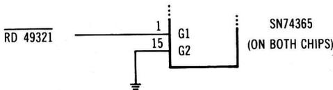
Fig. 3-11. Alternate control scheme for SN74365 three-state chips.
