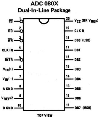
Fig. 6-23. Pin configuration of the ADC0804 A/D converter.
