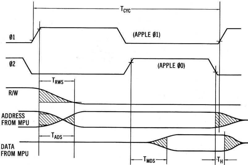
Fig. 1-4. Write operation signal relationships. (See Appendix C.)
