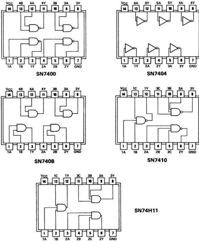
Fig. 2-1. Inverter and various AND/NAND gate pin configurations.
