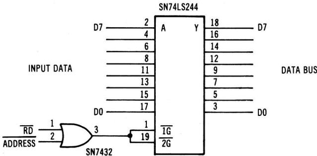
Fig. 3-12. Input port configured with an SN74LS244 chip.
