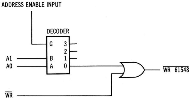
Fig. 2-9. Decoder used for absolute address selection.
