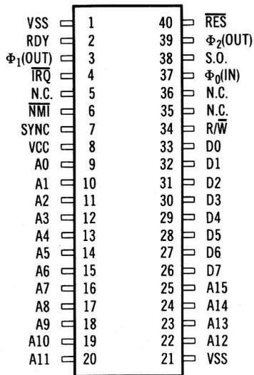
**Fig. 1-1. 6502 Microprocessor chip pin configuration.**
