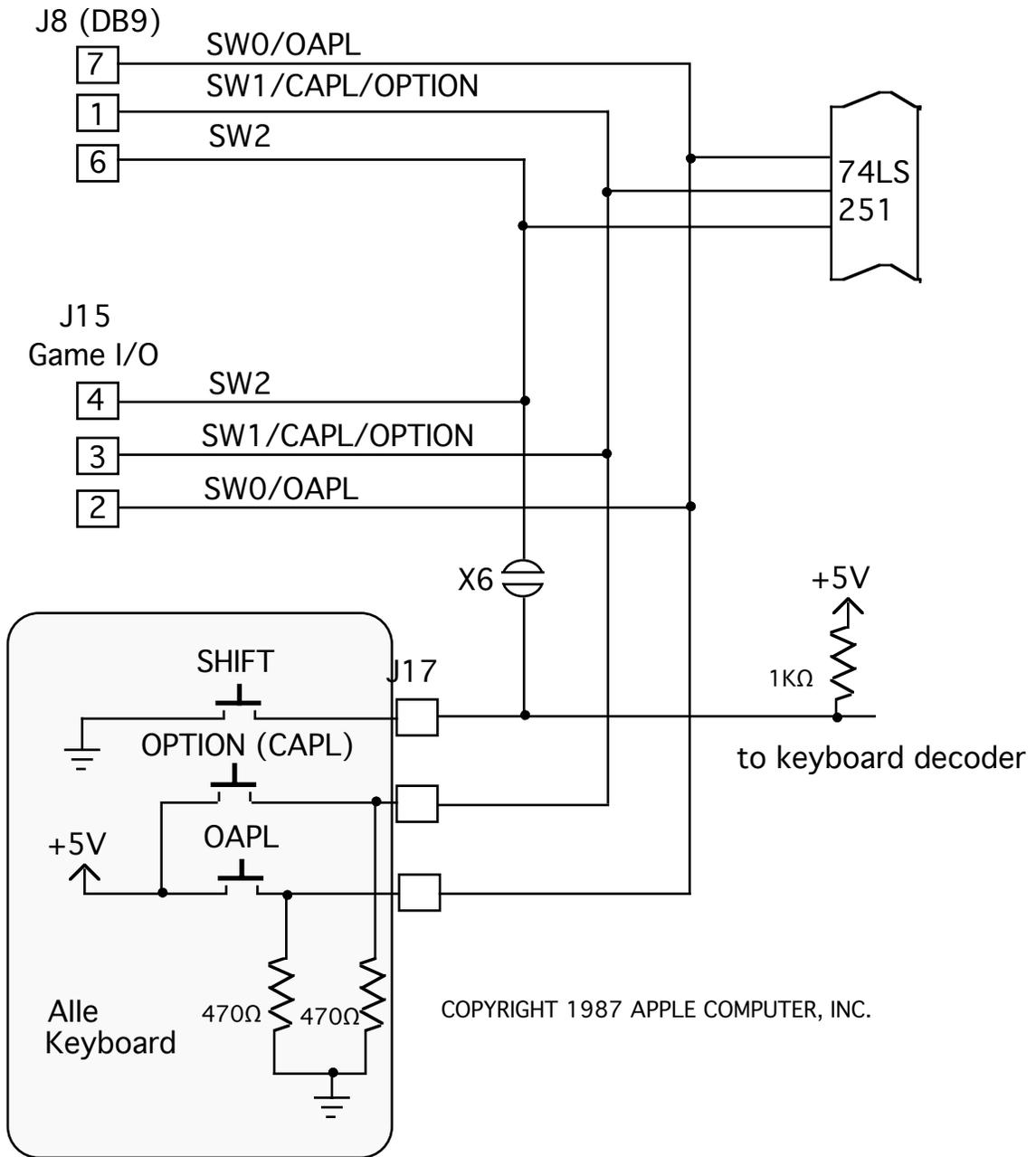
**Figure 2—Circuit for SW0, SW1, and SW2 (aka PB0, PB1, and PB2)
