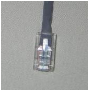
FIGURE 1.3 No Hood Cable
