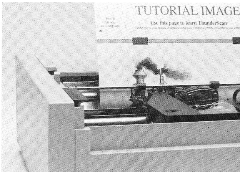
Figure 3.2 Proper position of original for scanning with an ImageWriter I or ImageWriter II. Note that the left edge of the original is lying even with the left edge of the platen.
