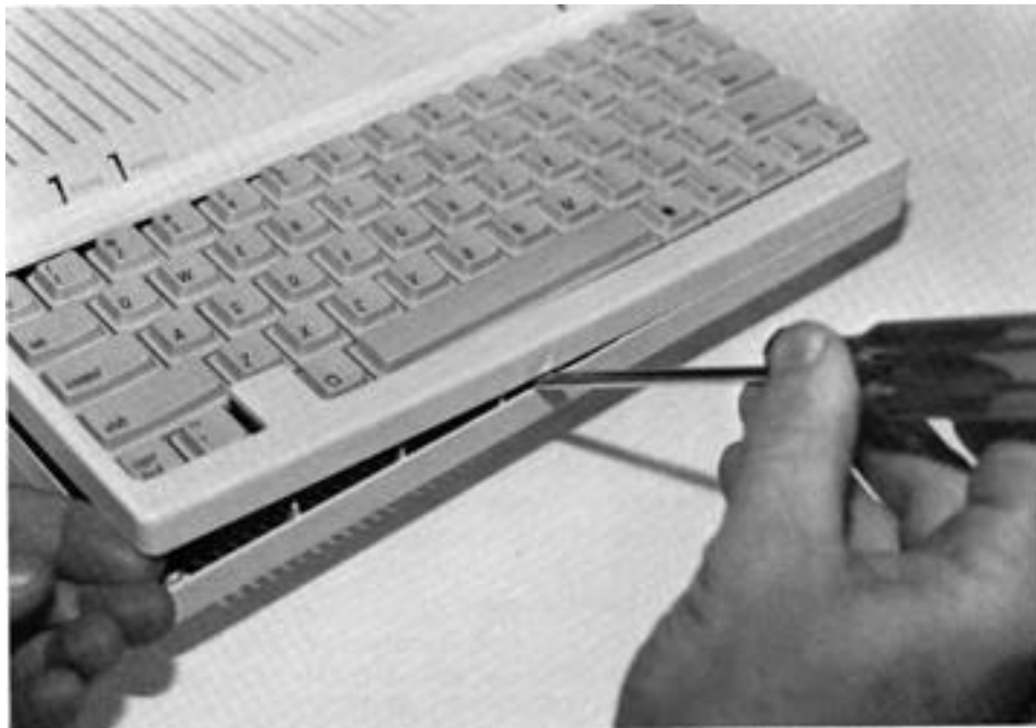
Figure 1-4. Releasing the //c keyboard bezel snap
