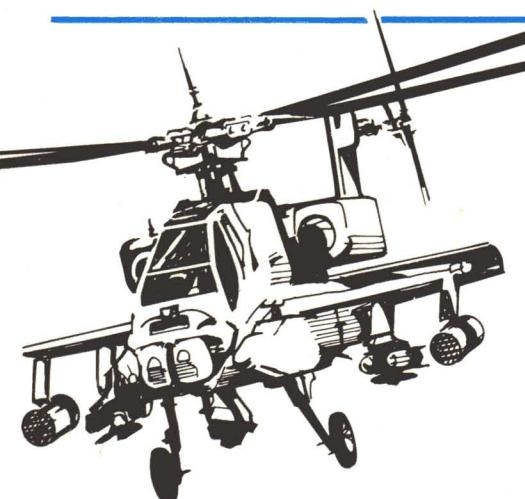
small "heads-out" display on his instrument panel. The TADS may be swivelled 120 deg right or left, 30 deg up, or 60 deg down. FLIR (Forward Looking Infra-Red) is used for night time vision, Daytime TV (DTV) in the near infra-red band can penetrate smoke and haze, and Direct View Optics (DVO) give a coloured display with a maximum magnification of  $\times 126$ —capable of visually zooming-in on a target up to 3 miles away! All three systems have a choice of field of view.
