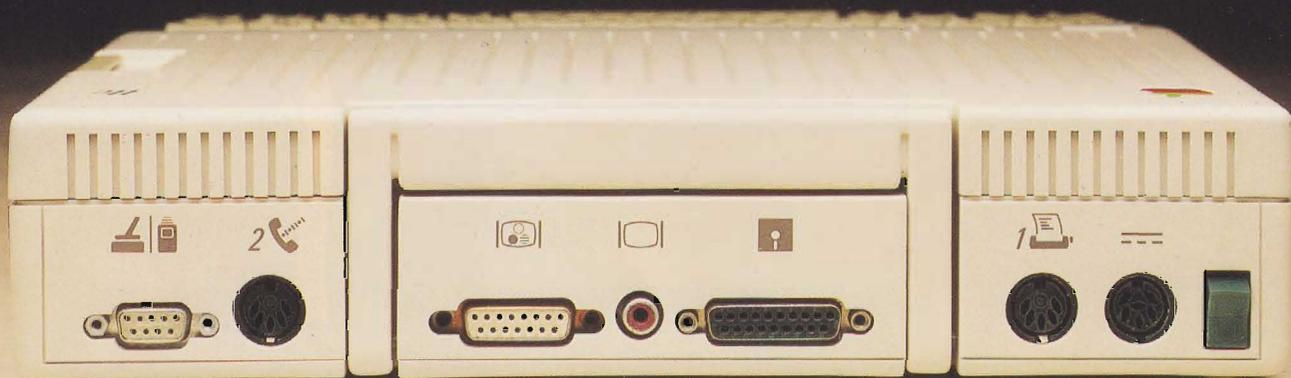
Mouse, Joystick, and hand controllers. Modem.
