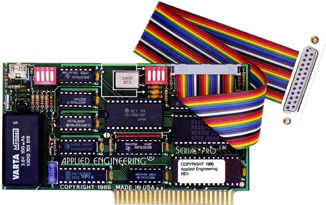
Serial Pro is a powerful multifunction card for the Apple IIe, II+, IIgs and Franklin computers. Serial Pro combines a powerful serial port for interfacing to either a printer, or a modem or other serial device, with a full function clock/calendar card. Serial Pro's serial port is compatible with virtually all letter quality and dot matrix printers, including Apple's Imagewriter and Imagewriter II. The serial port can communicate with the fastest external modems at baud rates from 50 to 19,200.
