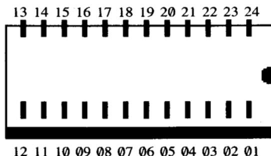
Your soldering skills come in handy now. Using some short, hi-gauge wire (wire-wrap is preferable, but anything in the 26-30 gauge will work), solder a piece between pins 21 and 24 and then solder a piece between pins 12 and 18.
