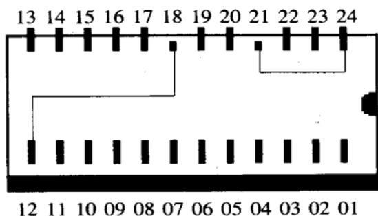
Double-check your soldering and the connections to be certain that pins 18 and 21 are cut off.
