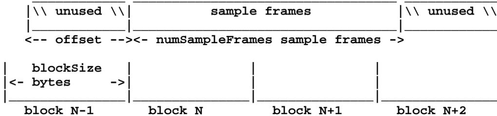
Figure 5-Block-Aligned Sound Data
