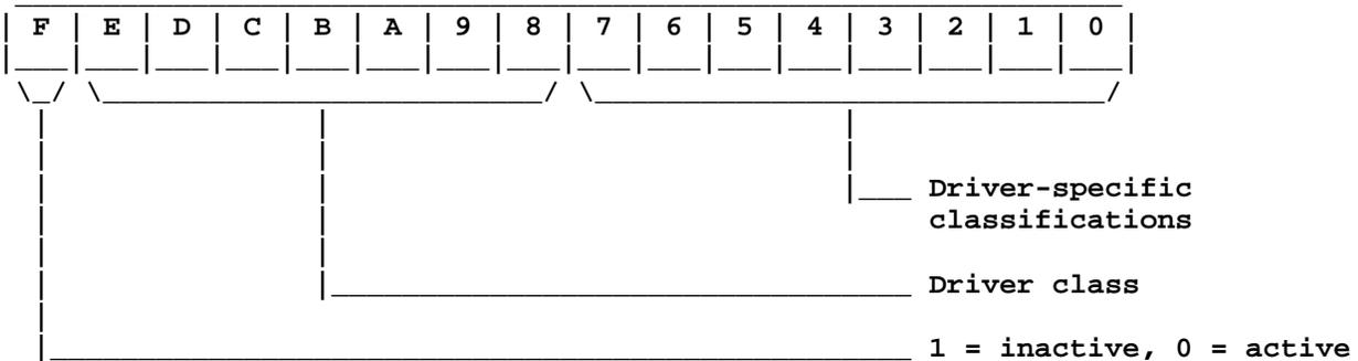
Figure 1-Auxiliary Type Definition
