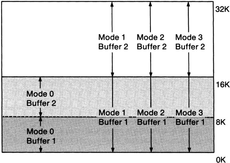
In a 128K Apple III, the entire 32K display buffer space shown is available for graphics. For any given graphics mode, the two display buffers occupy separate areas of memory, so that you can switch back and forth between their independent images. Also, both of the mode 0 display buffers occupy separate areas of memory from display buffer 2 of any other mode. This means you can switch between independent images in mode 0's buffer 2, for example, and mode 3's buffer 2.
