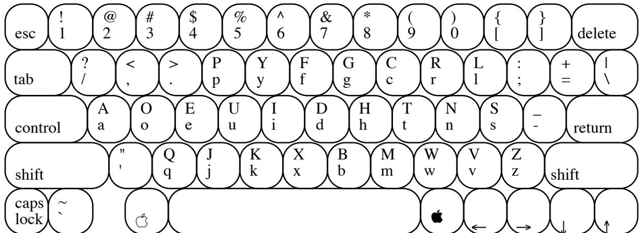
**Figure 1—Dvorak DSK Layout on Early IIc Computers**
