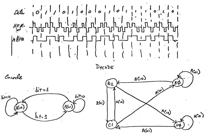
Figure 2-2. MHFM and HFM Transmission Codes.
