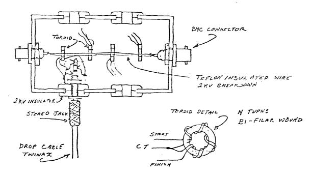
Figure 2-6. Applenet Node Connections.
