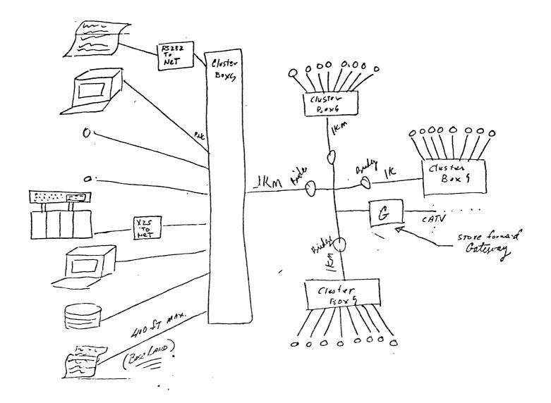
Figure 4-2. Baseband Network With Broadband Access.
