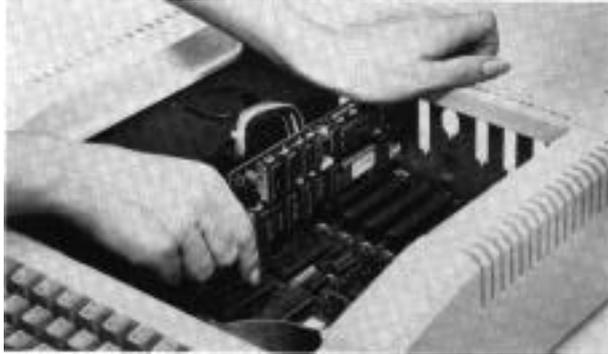
**Insert Controller Card into Slot**
