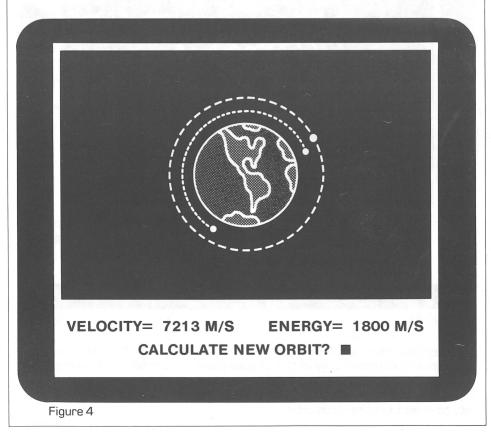
able energy is always given in terms of the amount of velocity change which can be accomplished. Indicate that these parameters are acceptable, and the new trial orbit will be plotted.
