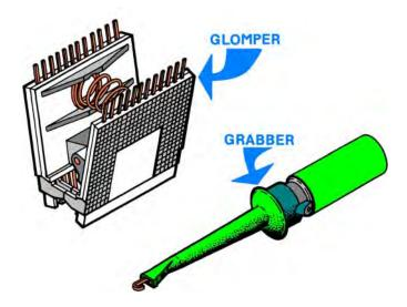
Glomper clips snap onto an integrated circuit and bring out all the pins to where you can conveniently reach them for very easy measurement or scope viewing. Grabbers are hook clips that let you safely catch one lead of an integrated circuit or another small component without shorting adjacent pins. **AP Products** is one manufacturer of glompers, while **E-Z Hook** supplies many of the grabbers. Selections of these appear in most new-age electronic distributor catalogs.
