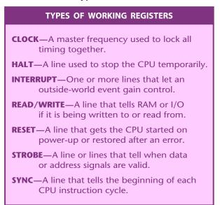
Once again, the object of a control bus is to use as few lines as possible to control the response of the microprocessor chip, the address space, and any interaction with the outside world. While most control lines go from CPU to address space, a few, such as the interrupt lines, may go the other way.
