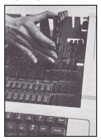
Inserting the Controller Card
