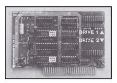
Now look at the new PROMs. The new PROM P6A should be marked 'P6A' or '341- $\emptyset\emptyset28$ -xx', or both. The new PROM P5A should be marked 'P5A' or '341- $\emptyset\emptyset27$ -xx', or both. You should be able to find these markings without peeling off any stickers. If you can't find the numbers at all, see your dealer.
