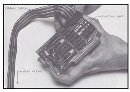
" Connecting the Cable to the Controller "
