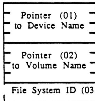
The D\_Info call has two parameters, a 2-byte device number that is inputted and a 4-byte pointer to a buffer that is also inputted. ProDOS/16 returns the device name into that buffer.
