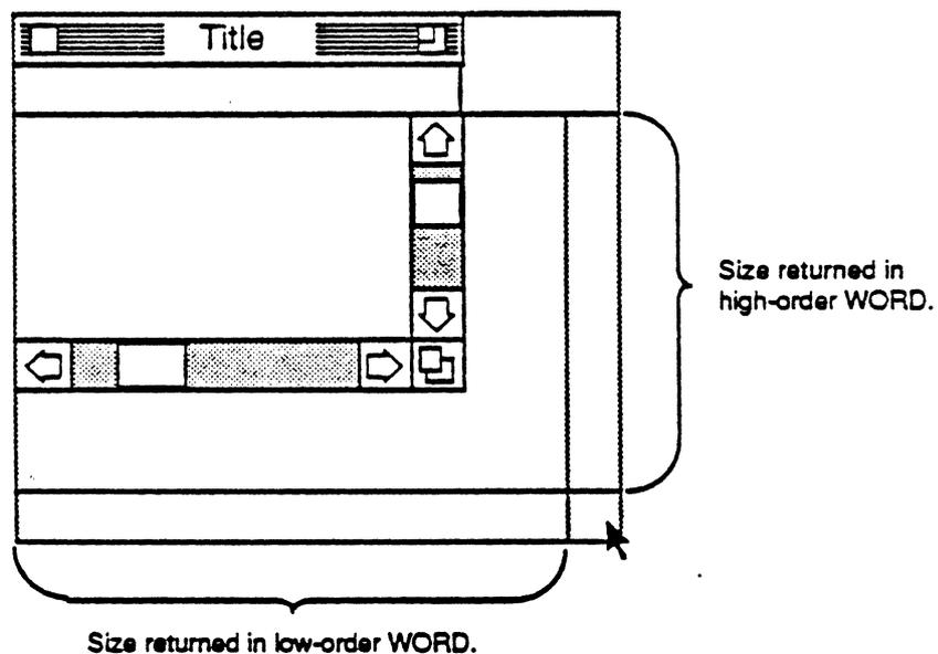
The application should subsequently call SizeWindow to change the portRect of the window's grafPort to the new one outlined by the grow image. The sizeRect parameter specifies limits, in pixels, on the vertical and horizontal measurements of what will be the new portRect. SizeRect.top is the minimum vertical measurement, sizeRect.left is the minimum horizontal measurement, sizeRect.bottom is the maximum vertical measurement, and sizeRect.right is the maximum horizontal measurement.
