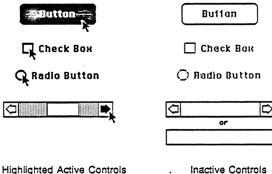
A control may be active or inactive. Active controls respond to the user's mouse actions; inactive controls don't. A control is made inactive when it has no meaning or effect in the current context, such as an "Open" button when no document has been selected to open, or a scroll bar when there's currently nothing to scroll to. An inactive is highlighted in some special way, depending on its control type. For example, the title of an inactive button, check box, or radio button is dimmed.
