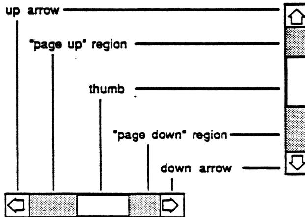
The parts of the scroll bars can be generalized into three regions; arrows, paging, and thumb (or thumber). The arrows scroll data a line at a time, paging regions scroll a "page" at a time, and the thumb can be dragged to any position within the scroll area. Although they may seem to behave like individual controls, these are all parts of a single control, the scroll bar type of dial. You can define other dials of any shape or complexity for yourself if your application needs them.
