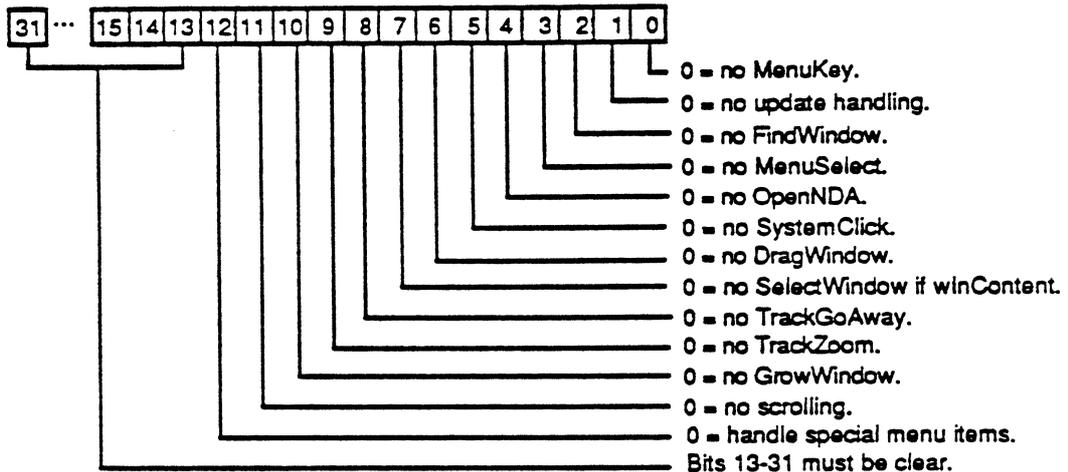
It is important that bits 13-31 be clear. In fact, TaskMaster will return an error if they are not. The bits are for future features which will continue to run with predated applications because bits 13-31 will mask off the new, unknown to current applications, features.
