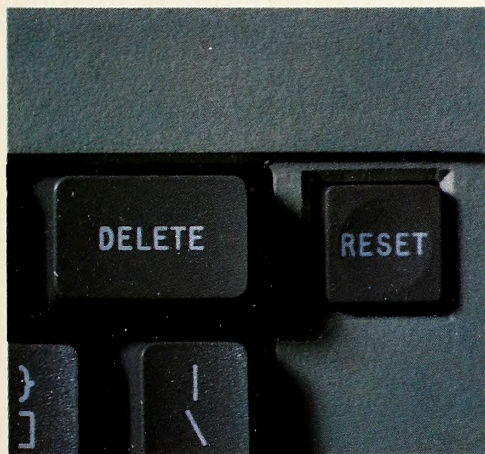
The new keyboard features a delete key. Note the reset key placed one step further out of harm's way.
